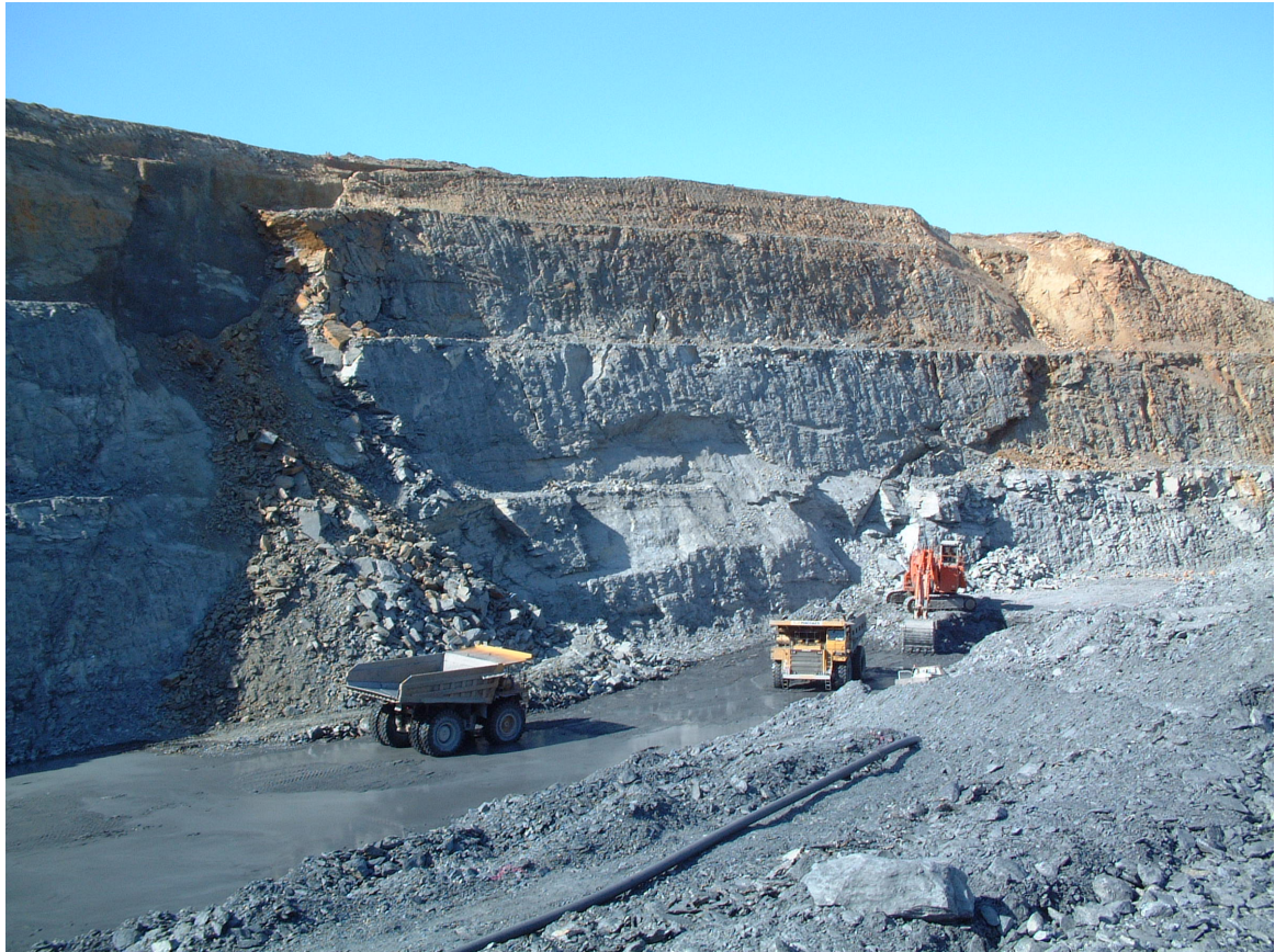
Photo 2 The presence of continuous structures within the Otago Schist is a certainty. GRD Macraes has, with PSM's assistance, established effective pit slope management guidelines to deal with mining under these adverse geological conditions.
